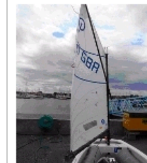
Fig.4 Outhaul not tightened
