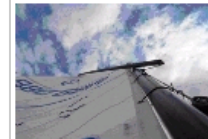
Fig.3 Luff too tight
